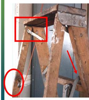
Ladders inspected frequently. Those with defects withdrawn from service for repair or destruction and tagged or marked as "Dangerous, Do Not
